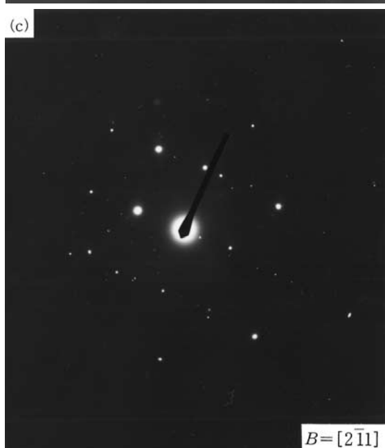
Figure 5 TEM micrographs showing reaction products, AlN: (a) BF, (b) DF, and (c) SADP in control alloy, and (d) BF, (e) DF, and (f) in the composite, respectively.
