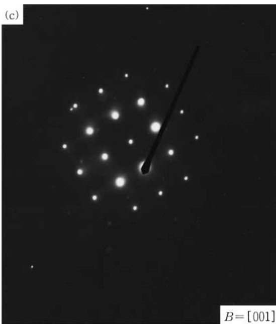
Figure 7 TEM micrographs showing reaction product, MgAl_2O_4 : (a) BF, (b) DF, and (c) SADP in control alloy, and (d) BF, (e) DF, and (f) SADP in the composite, respectively.
